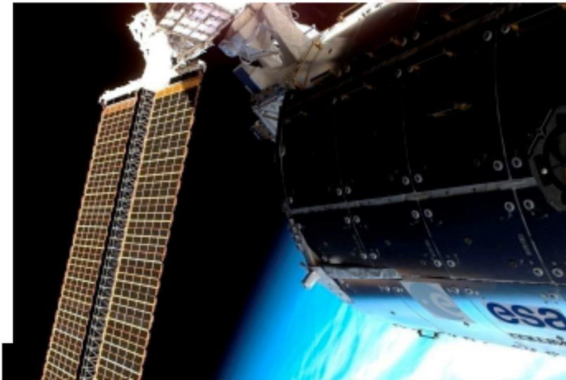
View of the European Columbus laboratory attached to the ISS
