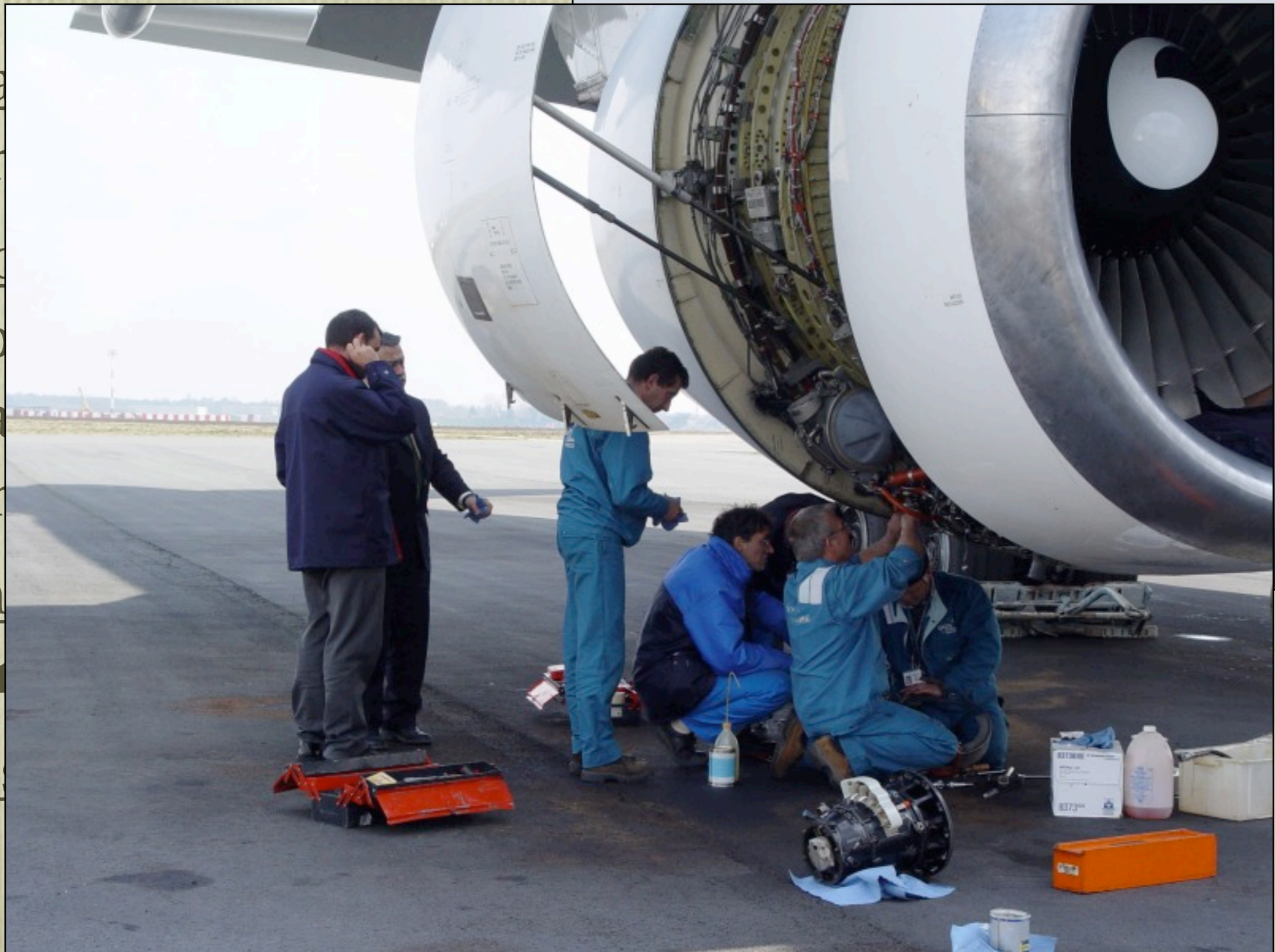
Exchange of the defect power generator
