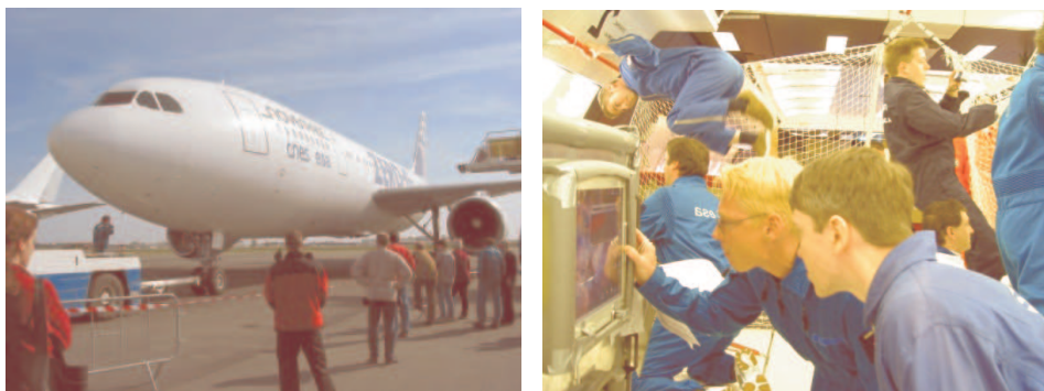
Fig. 8. The A-300 ZERO-G plane and the PK-4 experiment during the parabolic phase.
