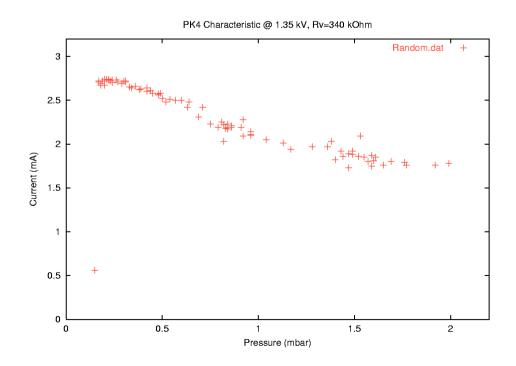
With the resistor of Rv=340 kOhm the tube voltage calculates to:
