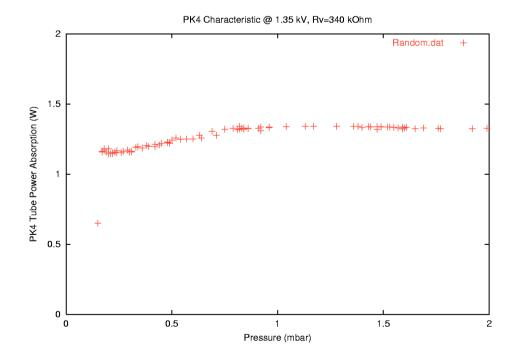
So, in contrast to the former 'leakage experiment' the power consumption of the discharge tube was roughly constant over the whole pressure range.
