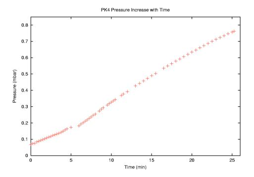
3.5 minutes after the experiment start, at a pressure of 0.137 mbar, the discharge ingnited spontaneously *with strong striations*. After 8 minutes (at 0.254 mbar) there was a sudden increase of the discharge brightness.
