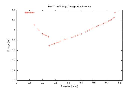
So, the power consumption of the tube in this 'leakage experiment' was:
