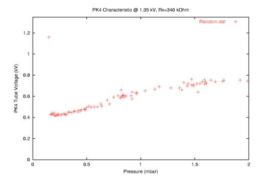
This results in a power consumption of the tube:
