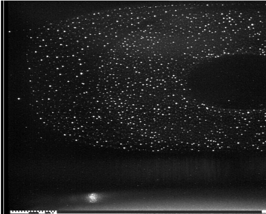
**Figure A.1:** A picture as recorded by the cameras in the PK3 plus setup. On the lower edge the format number can be seen.
