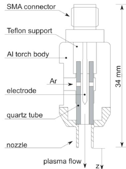
Fig. 1 Sketch of the plasma torch. Plasma is produced between the tip of the electrode and the surface of the quartz tube.
