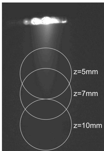
Fig. 3 Side view of the plasma flow. The exposure time was 30 s and the circles show the field of view for the optical spectroscopy measurements.
