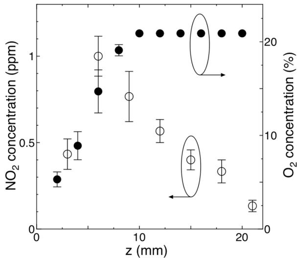
Fig. 2  $\text{NO}_2$  and  $\text{O}_2$  concentrations as a function of the distance from the torch ( $z$ ).
