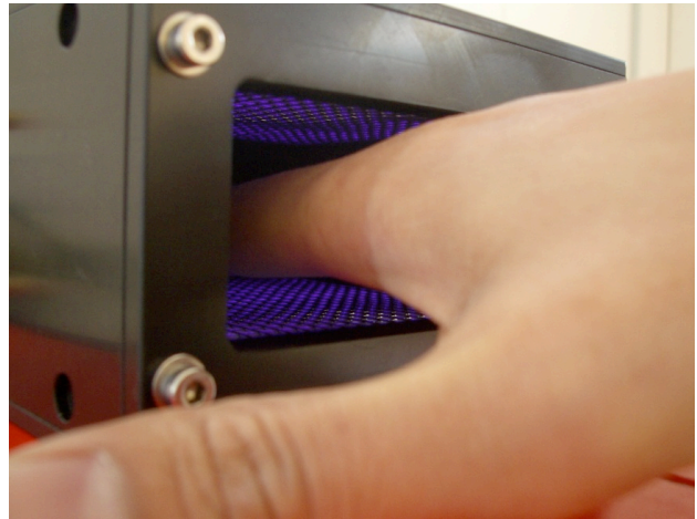
Fig. 1. Plasma dispenser. The plasma was produced on both electrodes with a voltage of 18 kV.
