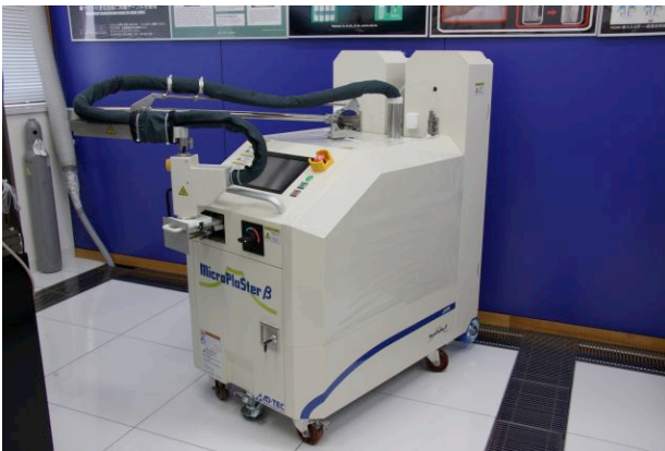
Fig. 2. The clinical device for wound treatment. At the end of the flexible arm the plasma torch is placed.
