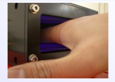
frequency: voltage: power: area: 12.5 kHz (sinusoidal) 15~18 kV<sub>pp</sub> 0.5 W/cm<sup>2</sup> ~100 cm<sup>2</sup> for each
