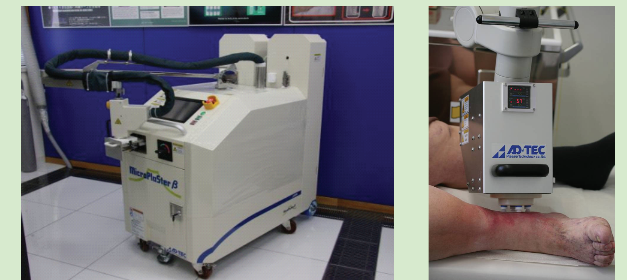
Microwave Plasma Steriliser \beta – argon plasma device for chronic wound disinfection
