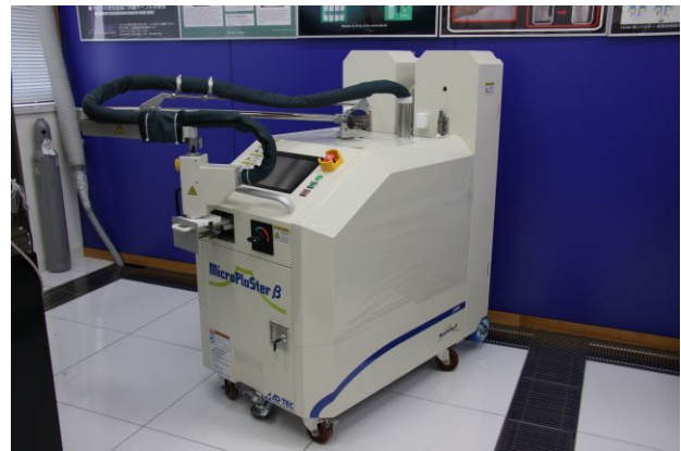
Figure: The clinical device for wound treatment. At the end of the flexible arm the plasma torch is placed.
