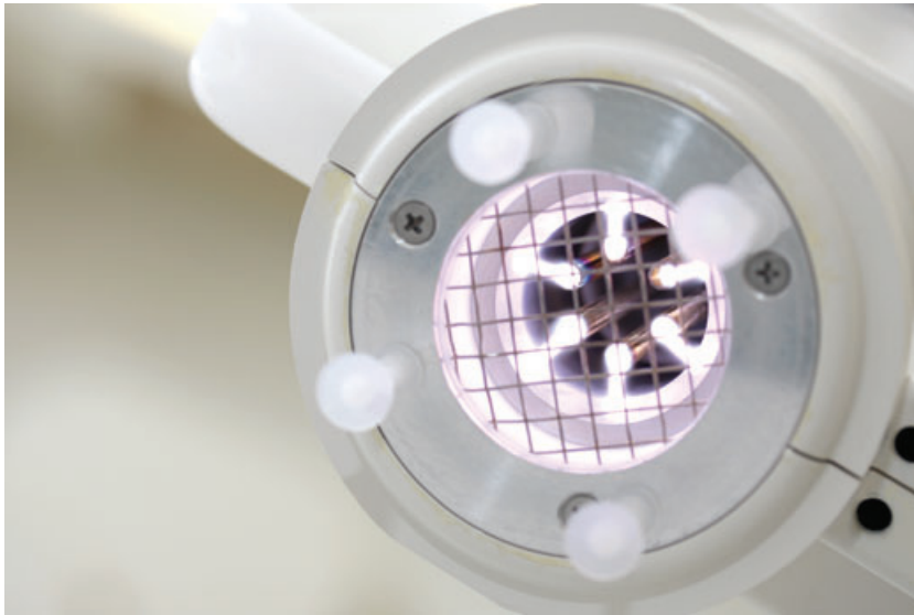
Figure 2: The plasma torch (MicroPlaSter \beta^{\circledR} ; 2.45 GHz, 86 W, Ar 2.2 slm) as an example of an indirect plasma source: Plasma is generated at the 6 electrodes and then transported to the target area via gas flow. The torch itself has to be cooled by air flow.
