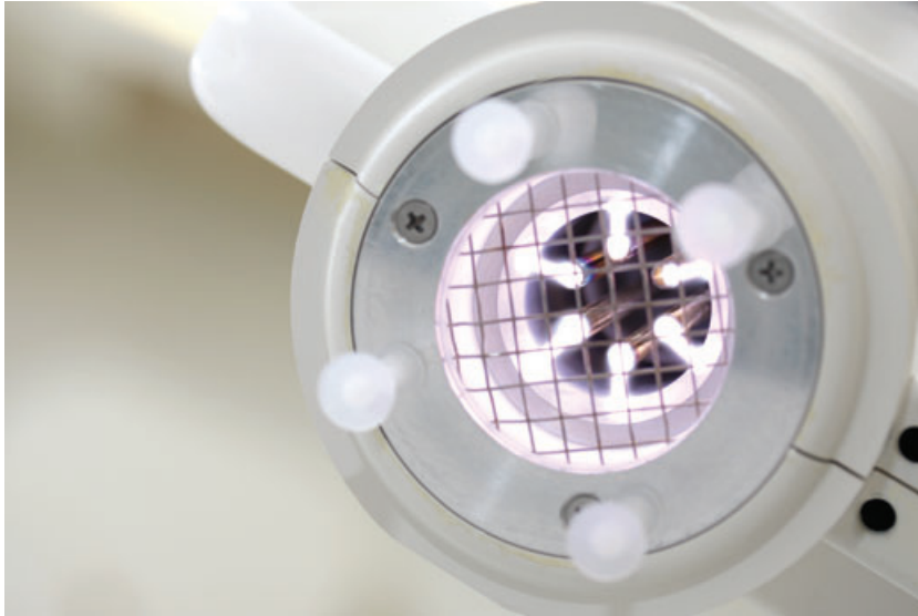
Figure 2: The plasma torch (MicroPlaSter \beta^{\circ} ; 2.45 GHz, 86 W, Ar 2.2 slm) as an example of an indirect plasma source: Plasma is generated at the 6 electrodes and then transported to the target area via gas flow. The torch itself has to be cooled by air flow.
